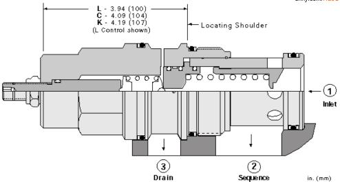
Pilot-operated, balanced piston sequence valves will supply a secondary circuit with flow once the pressure at the inlet (port 1) has exceeded the valve setting. The pressure setting of a sequence valve controls the pressure at port 1 relative to the pressure at the drain (port 3). These valves are insensitive to back pressure at port 2 (sequence), up to the valve setting. They may be used to regulate pressure in place of 2-port relief valves if there is pressure in the return line.
